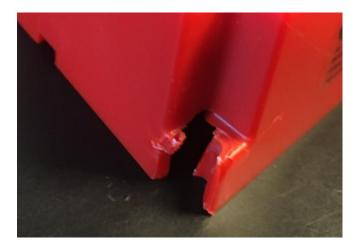
If using a threadlocker product such as Loctite®, it is critical that all excess threadlocker or spillage is cleaned from plastic after application. A damp towel or rag is the best way to achieve this. If excess threadlocker is not cleaned up right away, it could lead to damaged plastics.
